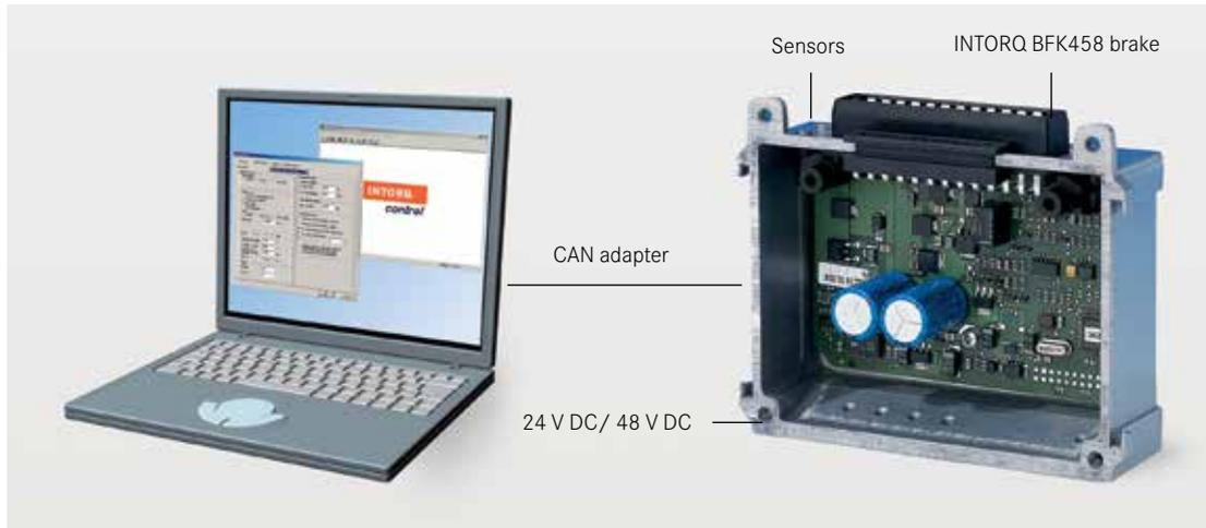
The mechatronic braking system is suited for controlled braking in battery-driven vehicles. The combination of a spring-applied brake with an intelligent control provides an optimal load-dependent braking torque (load-independent stopping distance). The control range covers 20 % to 100 % of the rated torque.
